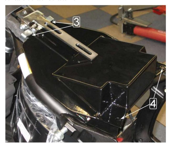
Push the square nut into the rack downside your seat. Mount the front part of the seat to the frame joint, loosely.
