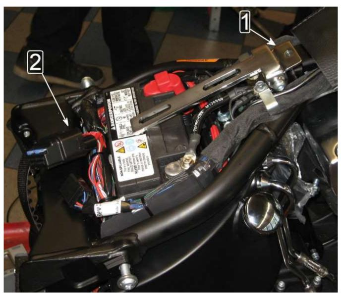
Remove the battery, then remove the complete plastic box and mount the battery again.
