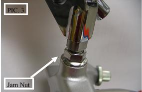
STEP 6 Holding the adapter with a wrench in adjusted position, tighten jam nut to the stock mirror
