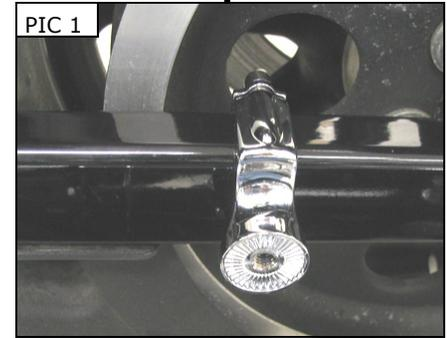
**ATTENTION!** DO NOT over-tighten the clamp! Over-tightening of the clamp could cause distortion and or breakage of the clamp. Kuryakyn will not issue a warranty on components that show signs of over-tightening.
