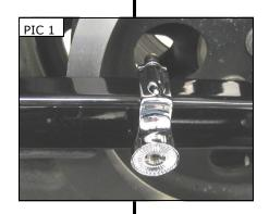
ATTENTION! DO NOT over-tighten the clamp! Over-tightening of the clamp could cause distortion and or breakage of the clamp. Kuryakyn will not issue a warranty on components that show signs of over-tightening.
