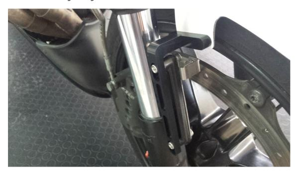
Now we must route the sensor cable along the front brake line. We can use a couple of plastic zips to hold the cable to the fork, and then route it along the front brake line using plastic zips or insulating tape.
