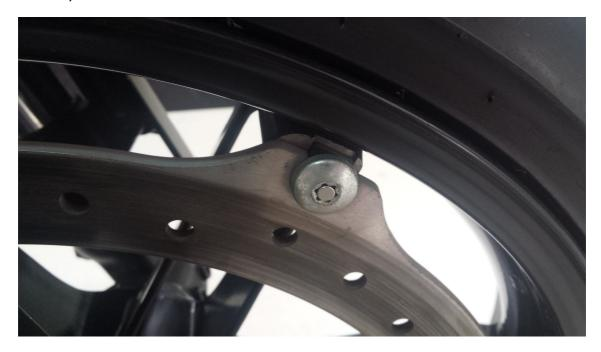
Once we have the magnets in place, we can mount the sensor. To do it, we must clamp the sensor bracket as next image shows, using the 2 short bolts.
