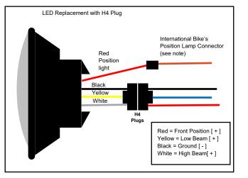
**Note:** The Red (position light or city light) wire is intended for international application which may require a position light to be illuminated in the headlight while the bike is parked on a street. It will be connected to the accessory circuit (position lamp connector) of the bike's harness and will illuminate when the ignition is placed in the accessory position.
