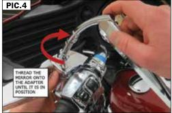
STEP 8 Adjust the mirror stem to your liking; use a 13MM wrench to tighten the jam nut down against the lever mount; use a 12MM wrench to hold the adapter in place while the jam nut is being tightened.
