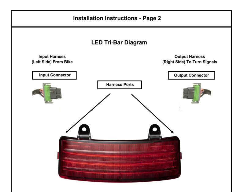
Plug the harness connectors into the new Tri-Bar, noting the rectangular ports on the back side of the unit. Left side should be going to the bike, the right side is the output to the turn signals. Make sure that the connector orientation is correct going into the ports, they are keyed one way, if the connector does not want to snap in, flip it around and try it again.
