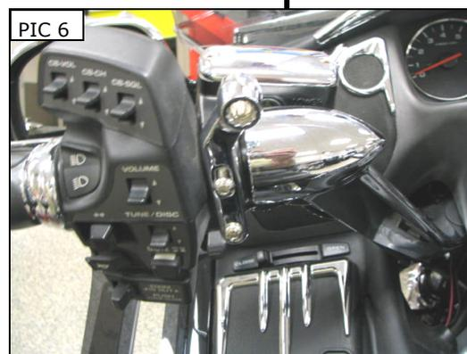
**NOTE:** For best results keep "L" shaped foot portion of the Tech-Connect Holder on the bottom of the device. Keep the device holding support arms centered on the mounting plate.
