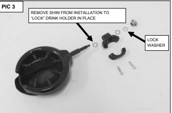
**STEP 6** Once you have the Drink Holder in the desired position, ensure that it will not interfere with the proper operation of the motorcycle by turning the handlebars to their full stop positions in both directions. Tighten all hardware.
