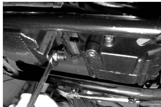
Tighten temp sensor with a 3/4" wrench
