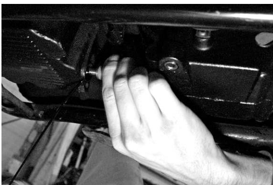
Thread sensor into oil pan
