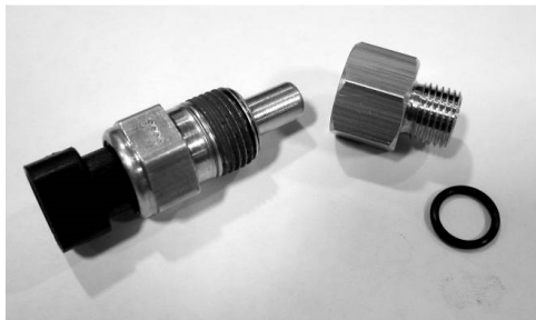
Assemble O-ring, brass adapter and sensor for 2017-up models prior to installation
