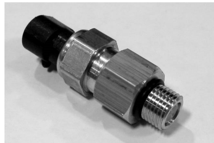
Assemble O-ring, brass adapter and sensor for 2017-up models prior to installation
