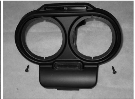
Gauges and gaskets removed
