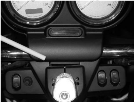
Tab (switch cover removed)
