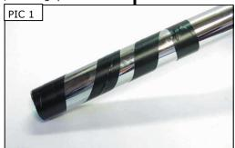
**STEP 4** Test fit each side. The throttle side grip has a slightly larger inside diameter than the clutch side grip. The grips should slide into place with slight resistance. If the grips slide on too loosely, make a "barber pole" wrap around the bar or throttle sleeve with electrical tape. PIC 1
