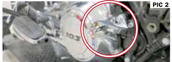
*Note: Pay attention to any spacers or washers installed between the male mount on the peg and the clevis. Placement of that hardware may be helpful later.*
