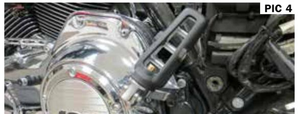
**WARNING** FOOTPEGS MUST BE INSTALLED SO THEY WILL FOLD UPWARD AND REARWARD IF HIT BY ANY OBJECT. FAILURE TO ADJUST THE FOOTPEGS TO OPERATE IN THIS MANNER COULD RESULT IN SERIOUS INJURY OR DEATH.
