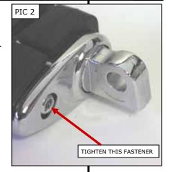
FOOTPEGS MUST BE INSTALLED SO THEY WILL FOLD WARNING UPWARD AND REARWARD IF HIT BY ANY OBJECT. FAILURE TO ADJUST THE FOOTPEGS TO OPERATE IN THIS MANNER COULD RESULT IN SERIOUS INJURY OR DEATH.
