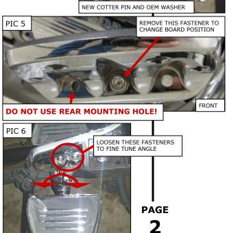
**COMFORT DROP MOUNTS/MINI BOARDS INSTALLATION**
