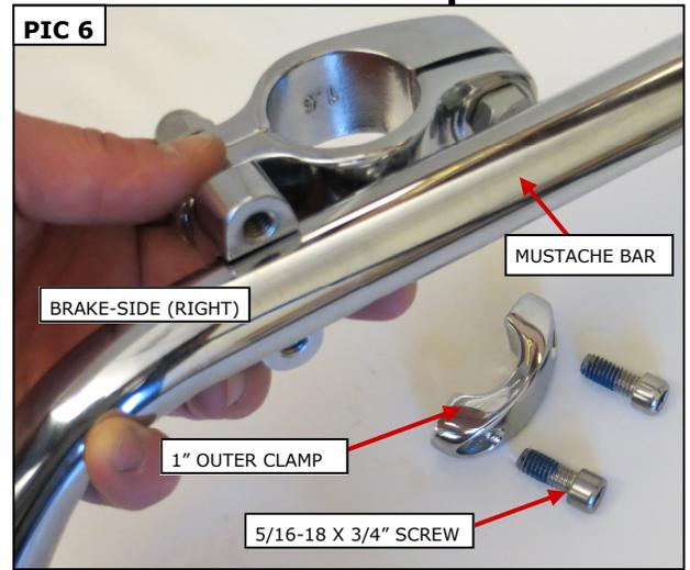
**STEP 12** Ensure the Mustache Bar is aligned correctly; tighten the fasteners starting with the 5/16" screws in the Outer clamps. Tighten the acorn nuts, then the hex head screws.
