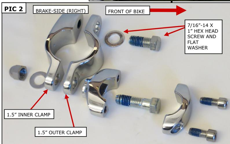
**NOTE:** The parts are shown disassembled and off of the bike for clarity. All parts should be installed on the bike as described in the following **STEPS**.
