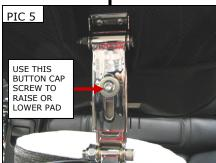
To raise or lower the Backrest pad, fold the pad up and slightly loosen the button cap screw on the post. PIC 5 Raise or lower the pad to the desired position, (there are detents inside the post that attaches the pad to the hoop that you may feel or here click as you move the pad). Tighten the button cap screw securely to lock the pad in place if you would like to maintain one set position.
