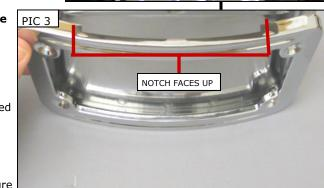
STEP 5 Fasten the license plate bracket to the light bar with the supplied 1/4"-20 X 1/2" fasteners.
