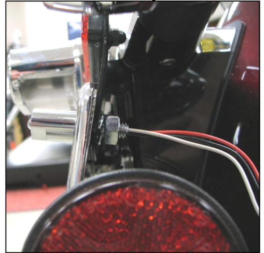
**STEP 3** Determine if you would like the RED L.E.D. Accent to operate with the running, turn or brake lights. Using the wiring schematic or a test light, determine the running light circuit to power the License Plate Illuminator's L.E.D. light. Determine a ground wire or source. Determine the power wire for the L.E.D. Accent—running, turn or brake.
