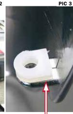
**SPACER INSTALLED TO** BACKSIDE OF TAB
