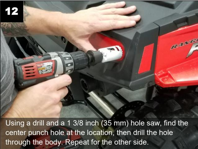
Using a drill and a 1 3/8 inch (35 mm) hole saw, find the center punch hole at the location, then drill the hole through the body. Repeat for the other side.
