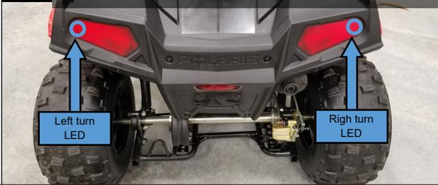
Decide where each Rear Turn signal will be mounted. The turn signal housings need a minimum of 1.8 inches of flat surface to properly mount. Note that the turns should be as far out to the corners as possible.
