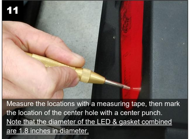
Measure the locations with a measuring tape, then mark the location of the center hole with a center punch. Note that the diameter of the LED & gasket combined are 1.8 inches in diameter.
