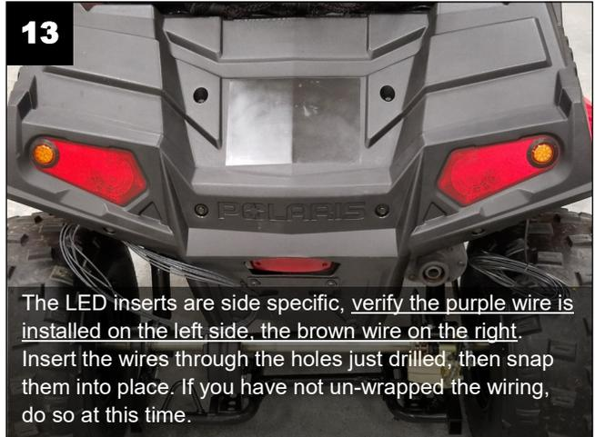
The LED inserts are side specific, verify the purple wire is installed on the left side, the brown wire on the right. Insert the wires through the holes just drilled, then snap them into place. If you have not un-wrapped the wiring, do so at this time.
