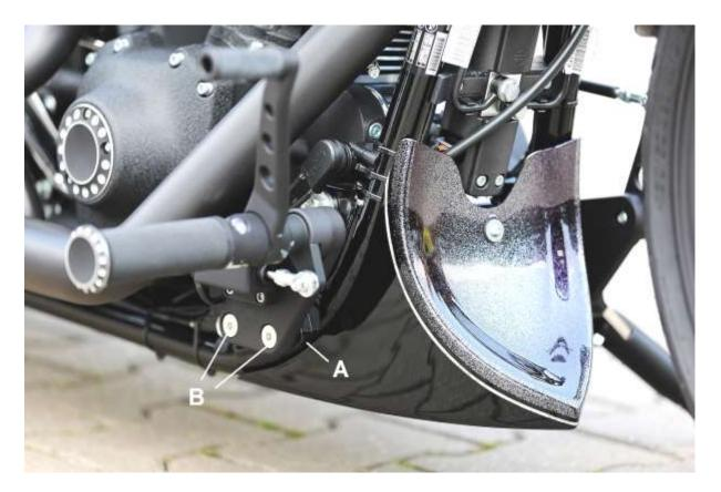
Place the spacers (A) between the frame and the backplate of the foot controls during the installation of the TB forward controls.
