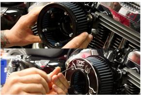
Apply anti-seize to threads of plug cap or v-stack and install hand tight.
