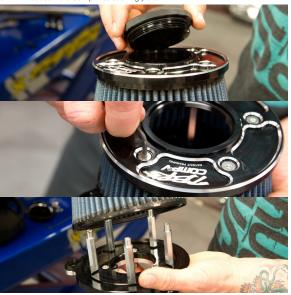
4. Install gasket onto back of backing plate.
