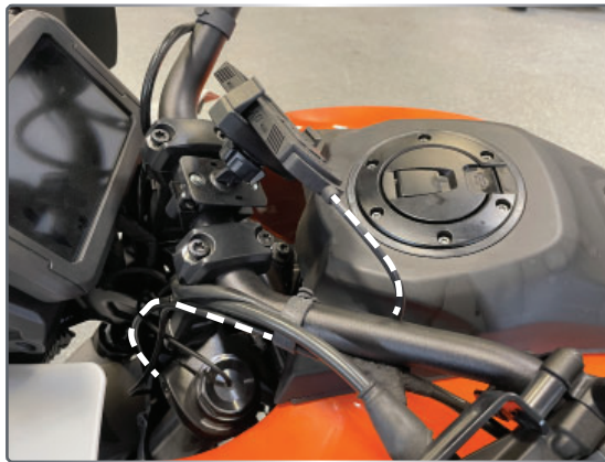
ROUTING THE CABLE
