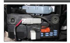
2012-2017 Dyna Models The diagnostic connector is located under the left hand side electrical cover. This connector is light grey in color with a black rubber plug installed.
