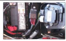
2011-2020 Softail Models The diagnostic connector is located under the seat attached to the frame by the rear fender. This connector is light grey in color with a black rubber plug installed.
