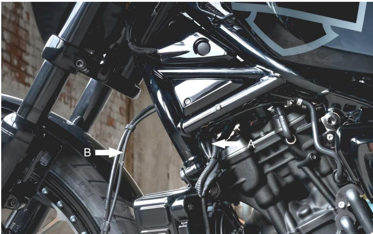
With this step you can also relocate the ABS sensor wire (B) to the inner side of the frame. There is a wiring connector underneath the upper left frame cover.
