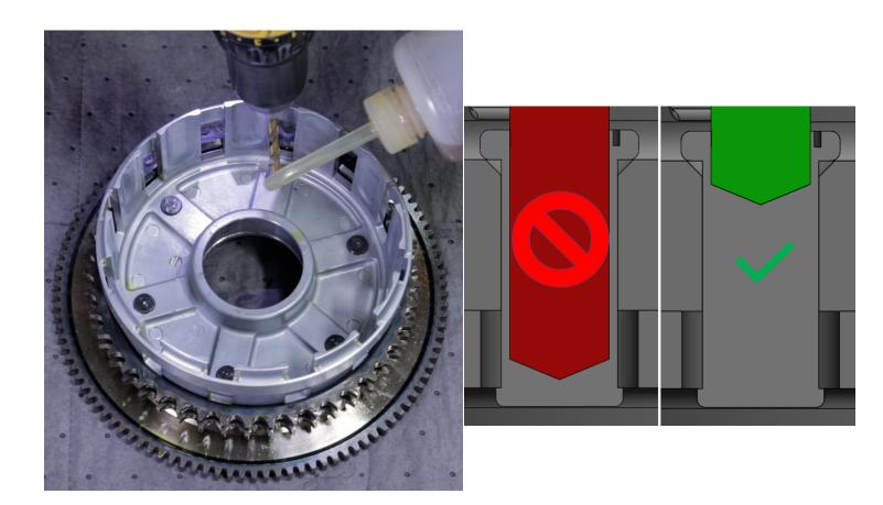
13. Remove the rivets from the basket assembly using a punch and hammer. Separate the ring gear and clean off any debris.
