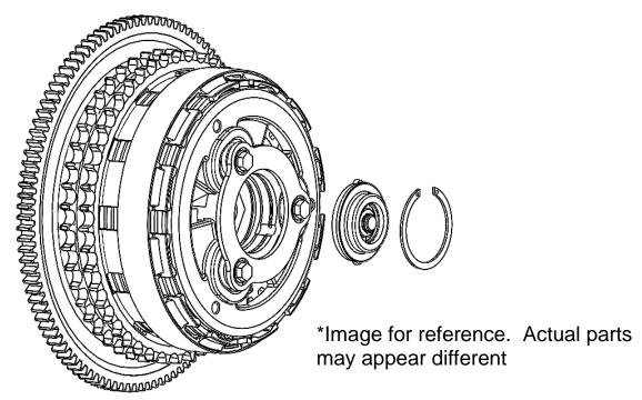
**Note:** If Rekluse RadiusX is installed, the clutch assembly will have to be disassembled during this step, do not remove the throw-out assembly.
