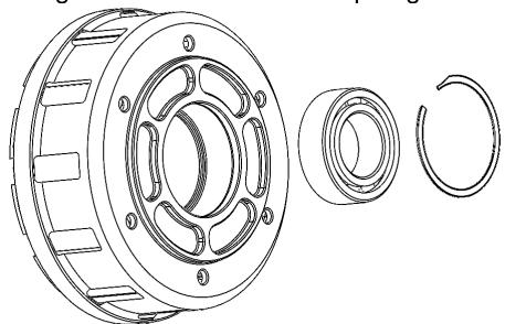
16. Assemble the Rekluse basket to the ring gear using the supplied hardware. Use included Loctite and torque nuts to 80 in-lbs (9 N-m).
