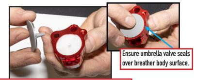
Install umbrella valve and disc on top of filter element.
