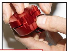
Install cover onto breather body. Apply 263 loctite onto button head fastener before threading into cover
