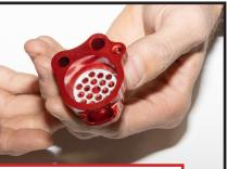
Install lower perferrated disc (smaller) into breather body. Make sure disc is flat and fully in place inside housing
