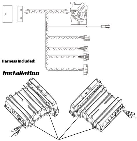
Use OEM head unit mounting locations & original screws
