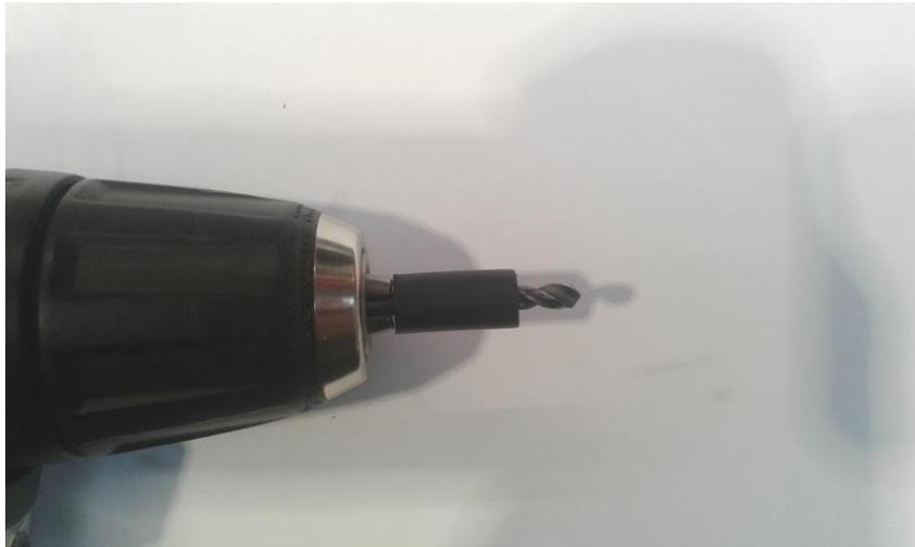
Drill both outer holes into your seat pan for the rear bracket.
