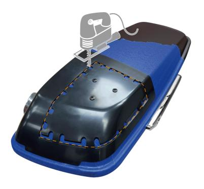
**5.7.1** Follow the cut line around the drilling template (see the dashed orange line in the image above), cutting through the plastic tabs as you go. The kit allows for some tolerance in the cut, so precision is not critical. **However, a perfect cut will allow the central part to be removed without trimming.**
