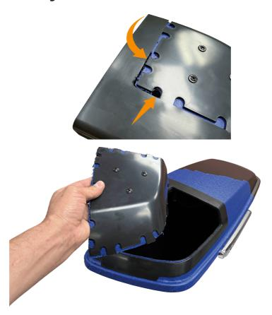
Be careful not to let the tool jump out to avoid damaging the cover. Using a variable-speed jigsaw is essential for good control.
