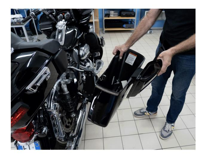
**5.1.2** To facilitate the wiring, unfasten and remove the side cover by pulling it towards you as shown in the image.
