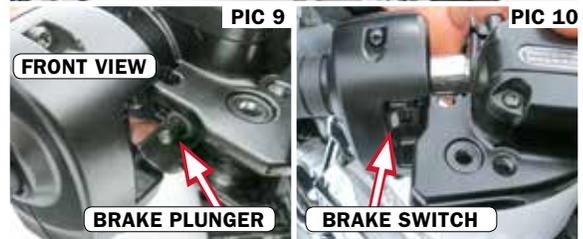
**STEP 12** Reinstall the pivot pin and secure with the snap-ring. Tighten the brake (right) side handlebar switch housing assembly screws. Compress the Brake Lever a few times to ensure that the brakes works properly BEFORE starting the motorcycle.
