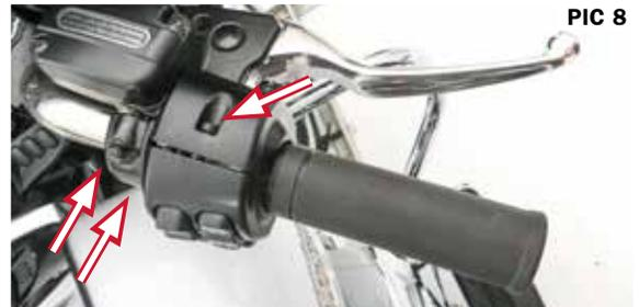
**STEP 9** Refer to PIC 8. Loosen the screws securing the brake (right-side) handlebar switch housing assembly.
