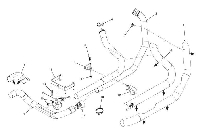
NOTE - Install #18 heat shield clamps with screw heads pointing in direction shown by arrows.
