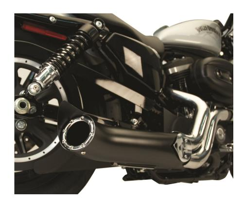
Phantom Pipe™ by Paul Yaffe Baffled, Black Ceramic 2:1 Drag Pipe with Chrome Heat Shields.
