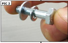
Refer to PIC 2. Insert the four included 1/4" Screws, Lock Washers, and Flat Washers through the support frame and into the Tour Pak™ floor. Leave the screws loose until all four have been started in their threaded holes.
