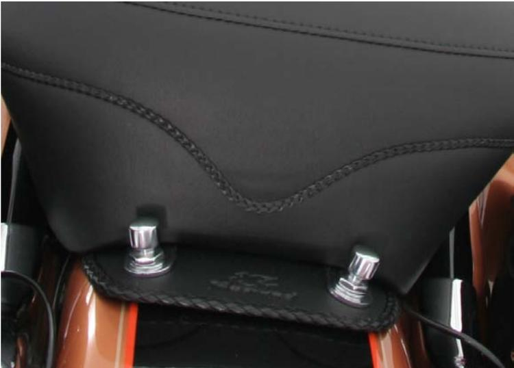
5. Place the nylon shoulder washers (1999-2007) or flat washers (1997-1998) on the fender studs and then put the rear mounting tabs over the studs.
