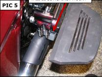
**On `10-'14 trike applications: Refer to PICs 2 through 5.** Locate the included Stop Bushing marked "TRIKES"; install it on the brake-side (right) bottom-mount; install one of the other Stop Bushings on the clutch-side (left) bottom mount; ensure the taller edge goes against the top mount/pivot arm assembly.
