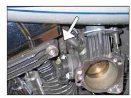
6. Using the provided tie wrap, secure the wiring pig tail to the throttle body wiring harness. NOTE: On non-US models, a by-pass module (sold separately) will need to be installed onto the pigtail to eliminate an engine management light from turning on. (non-US models only)
