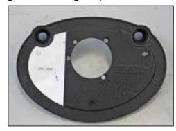
3. Remove the three bolts that secure the air filter to the filter base and remove the air filter along with the crank case breather tubes. 5. Remove the air filter base from the throttle body and unhook the wiring pig tail from the filter base. **NOTE: K&N Engineering, Inc. recommends that customers do not discard the factory air intake components.**
