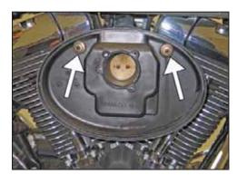
4. Remove the two crank case breather bolts shown.
