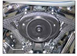
14. Install the air filter onto the base plate and secure with the three bolts provided. NOTE: Apply one drop of thread locker to each bolt.
