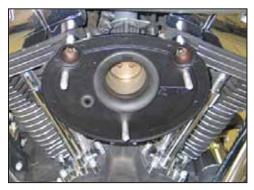
13. Install the base plate onto the throttle body and then secure with the factory breather bolts and throttle body bolts provided.
