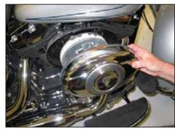
2. Remove the bolt that secures the bonnet to the filter assembly and remove the bonnet from the vehicle.
