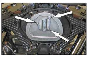
3. Remove the three bolts which secure the air filter to the filter base and then remove the air filter along with the crank case breather tubes.
