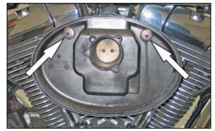
4. Remove the two crank case breather bolts shown.
