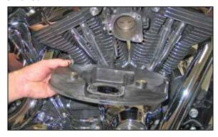
Remove the air filter base from the throttle body and unhook the wiring pig tail from the filter base.
