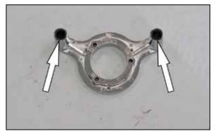
7. Install two of the provided o-rings into the K&N $^{\mbox{\scriptsize \$}}$  crankcase breather plate as shown.
