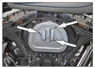
3. Remove the three bolts that secure the air filter to the filter base and then remove the air filter along with the crankcase breather tubes. **NOTE: The factory air filter may differ from the picture; it may also have a bracket attached.**  shown.
