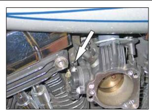
6. Using the provided tie wrap, secure the wiring
