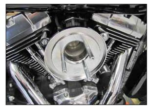
9. Install the three spacer/bolts into the K&N<sup>®</sup> filter base plate, then install the base plate gasket and one drop of thread locker onto each spacer/bolt. Install the K&N<sup>®</sup> filter base plate assembly onto the breather plate as shown.
