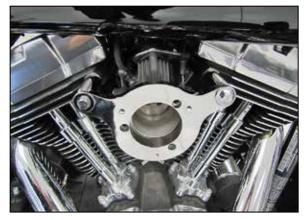
8. Install the K&N<sup>®</sup> crankcase breather plate along with the two remaining o-rings, mounting bolts (with one drop of thread locker) and the throttle body gasket as shown.
