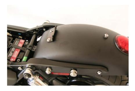
2. Place the seat onto the frame and slide it forward, engaging the nose bracket into the receiver under the gas tank.
