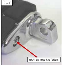
FOOTPEGS MUST BE INSTALLED SO THEY WILL FOLD WARNING UPWARD AND REARWARD IF HIT BY ANY OBJECT. FAILURE TO ADJUST THE FOOTPEGS TO OPERATE IN THIS MANNER COULD RESULT IN SERIOUS INJURY OR DEATH.
